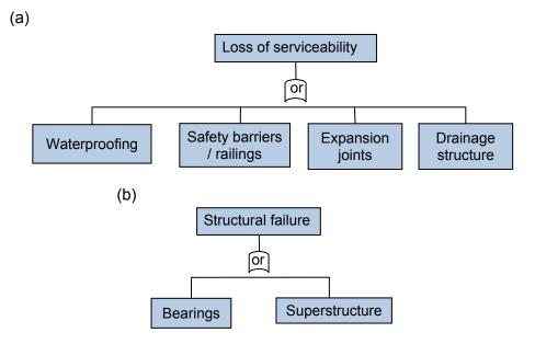
Figure 9. Fault tree model used for bridges (Danish case study) for (a) loss of serviceability and (b) structural failure.
